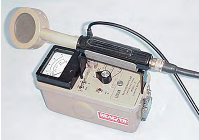
Radiation survey meter (GM meter). (Source: Steve Sugarman, REAC/TS.)
